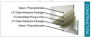
This product is manufactured using ANSI Z97.1 for laminated safety glass construction
